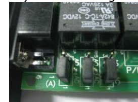
Fig. 6 Jumper setting for ACTIVE CLOSE
