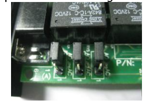
Fig. 7 Jumper setting for ACTIVE OPEN
